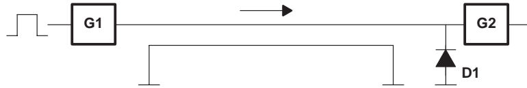
Figure 27. Typical Point-to-Point Connection
